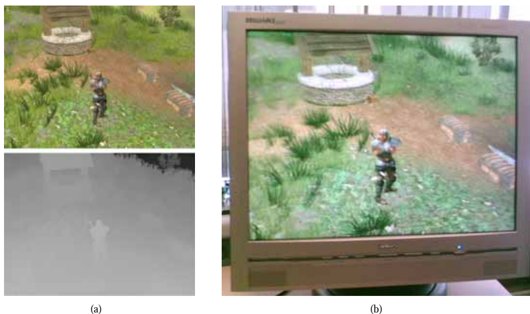
FIGURE 14: Screen shot of GOAL: image and depth buffers (a), and actual image on autostereoscopic 3D display (b).
